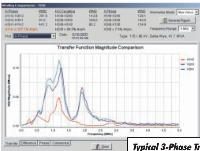
**Typical 3-Phase Transformer Transfer Function Plots with OWA Results Displayed**
